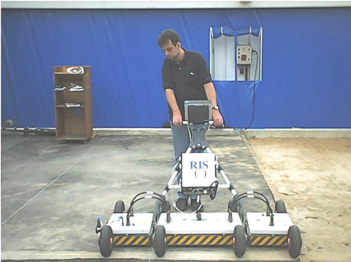
Figure 5: Data collection with the RIS 2K – MF configuration at the GDF test site
